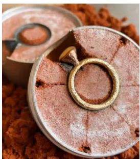
Casting silver is trickier than casting gold. There is less metal used in gold casting, and the sprue is smaller.
