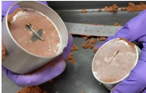
Sprinkle talcum powder or similar on top of the sand. This prevents the two halves of the sand-filled frame from sticking together. Not too much powder. Use a brush to cover the whole top side and remove the excess.
