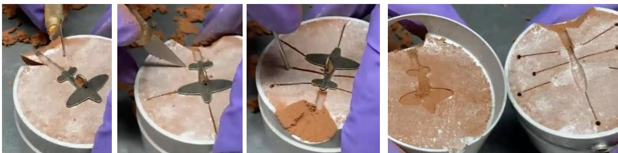
Re-connect the frame pieces and cut out the rest of the funnel. You do not want any loose sand that might be picked up when the metal is poured in. Finally, mark where the other half of the sprue will be. Take the frame apart and complete the sprue. Make sure the sprue touches the impression of the piece to be cast.
