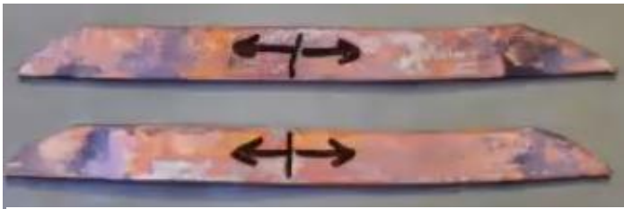
Two copper pieces folded and ready for forging, with the open edge upwards on both pieces. Hammering goes from the central line in the direction for the arrows.
