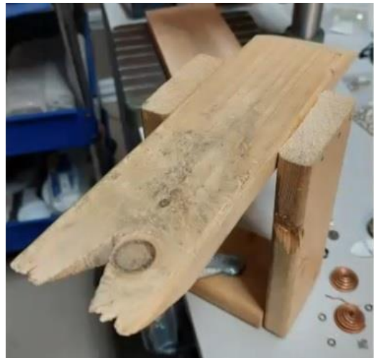
The Karl Bench Pin: raised bench pin for low tables, designed by Karl Schutt
