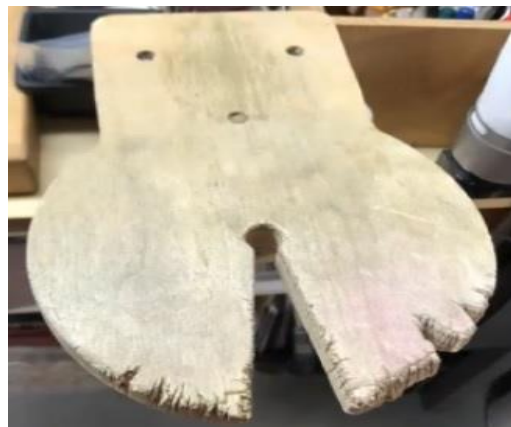
Bench pin used by Vicki Jasperse has a large work surface. It has its own stand that can be clamped to a table.
