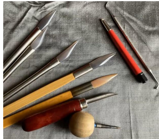
Photo of tools to apply gold foil including burnishers and dental scrapers.
