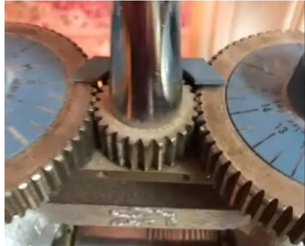
View of the calibration/measuring dials on the top of a rolling mill.
