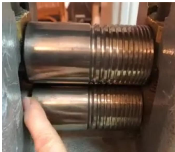
A trusty little Cavallin combination mill with a 50mm flat side and a grooved side.
